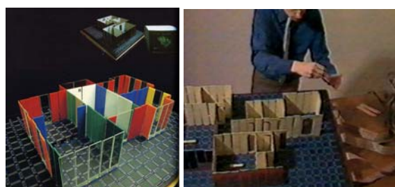
Fig.9 Self-builder design kit, working electronic system (left) and user demonstration (right) , designed by John and Julia Frazer, consultants, with John Potter, research assistant, for architect Walter Segal, 1982.
