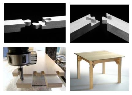
Fig. 2 a-d Digital wood joints, table with digital wood joints (design: Jochen Gros)
